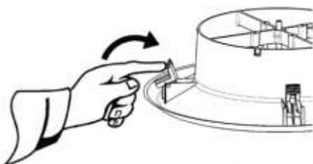
5. Carefully pass the grille up into the opening ensuring all clips are triggered down.
