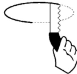
3. Pull the duct through the opening in the ceiling and attach the grille to the duct using duct tape.
