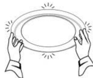
6. Adjust the air quantity by spinning the diffuser cone clockwise or anticlockwise - Clockwise to close
